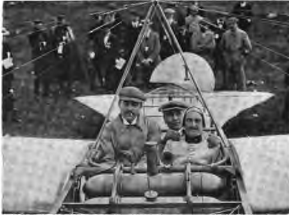
MORANE WITH TWO PASSENGERS ON HIS BLÉRIOT XI 2 BIS Note the framing, the fan-tail and the direction rudder at the rear.
